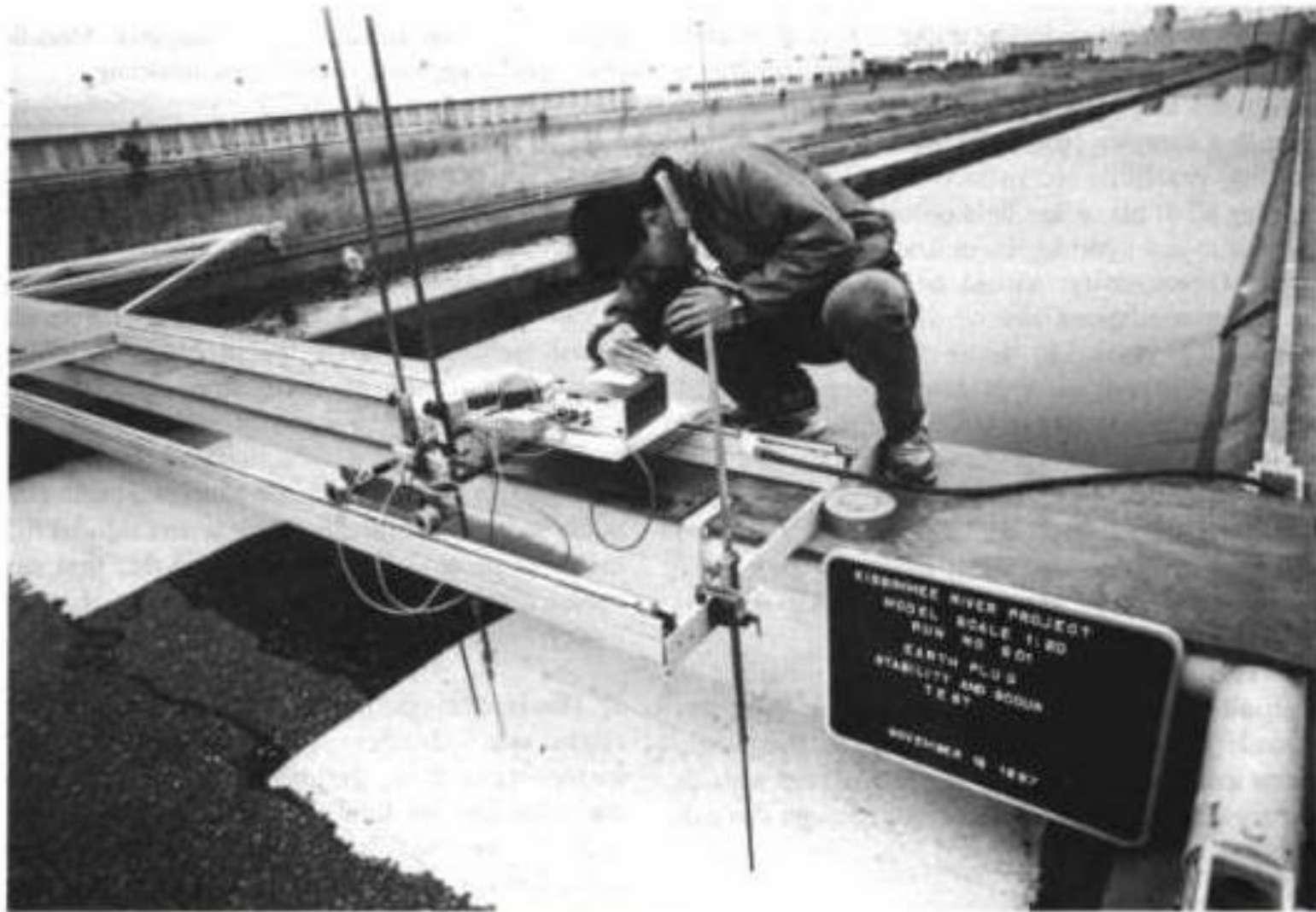
Figure 26-2b Physical Modeling. On the Kissimmee River restoration project, studies combined the use of physical and computer models. This photograph shows measurements being taken for an earth plug stability and scour test on a physical model constructed to a scale of 1:20. (photograph by Pat Partington, SFWMD)
